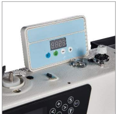
数控数字调节，时分分段打，一次可分9段。 Electronically controlled digital adjustment with time-segmented pleating capability (programmable up to 9 segments)
