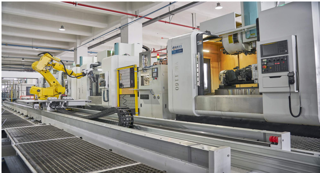
公司拥用3条机器人机壳机加工自动线 The production workshop consists of 3 automatic robot casing machining lines
