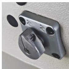
一步两点和三步四点转换装置 One step, two points and three steps, four points conversion device
