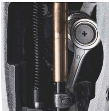
干式无油润滑, 镀黑金钢针杆 Dry and pollution-free lubrication Super wear resistance Plated steel needle rod
