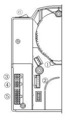
Motor socket ② Motor encoder socket ③ Pedal switch socket ④ LED light/ Backstitch switch
