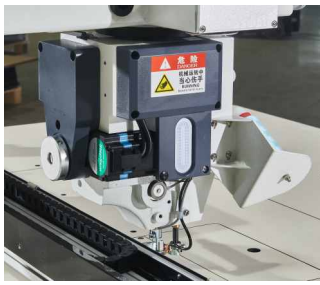
步进电机抬压脚,结构简单,易调节,对不同面料调整快,适应性广。 Stepper Motor Lift Presser Foot, Simple Structure, Easy to Adjust, Quick Adjustment for Different Fabrics, Wide Applicability.
