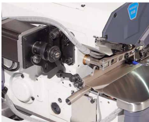
步进驱动，剪线，抬压脚 声音轻 Stepper adjustment of stitch length, presser foot lifting, thread trimming, sound light
