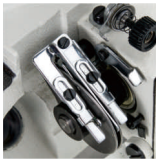
打线凸轮外置 (穿线、维修更方便) External cable & cam (More easy to thread & maintain)
