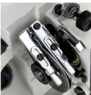
打线凸轮外置 (穿线、维修更方便) External cable & cam (More easy to thread & maintain)
