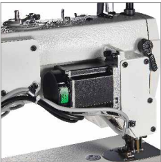
采用伺服电机驱动上差动压脚。 Servo motor-driven upper differential presser foot
