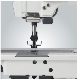
三档调节LED光源及补针 Three-stage adjustable LED light source and needle compensate
