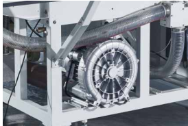
配备大功率高压旋涡风机，吸风效果强，噪音低 Equippped with High Power and Pressure Swirl Air Blower, Strong Sucking Effect,Low Noise, Partitioned Sucking Device Box, Flexible Switching for Suction of Fabrics.
