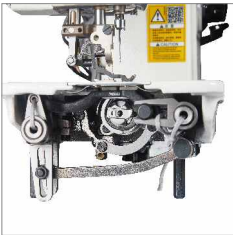
采用双牙架下差动结构。 Dual rack lower differential mechanism
