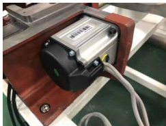
上下双伺服独立驱动，高速、静音、低振； Up and down double servo independent drive, high speed, quiet, low vibration;
